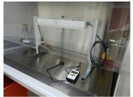
Figure 1. Lind Equipment UV-C Device in CL3 BSC.
